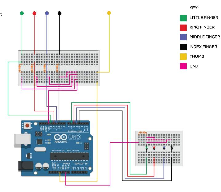
This is my initial glove controller concept, built from the diagram with everything connected together. Obviously I will extend the wires at a later date as they are not long enough but as a starting point this should work.
