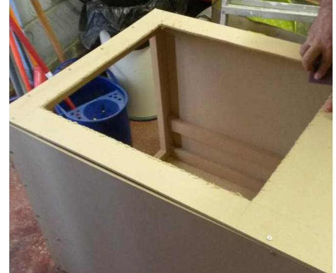
Step 9: A door was then cut into the back of the box for access later on.
