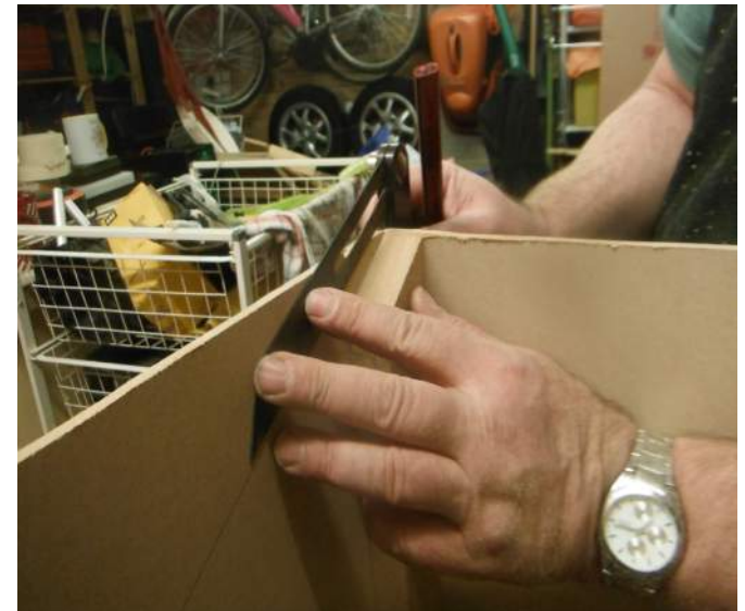
Step 6: The angle for the screen was then measured and timber beams were cut and screwed into place at the right angle.
