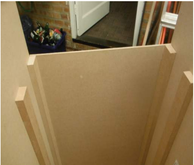
Step 4: Inside the box two more lengths of timber were put into place to indicate the place the console will rest on.
