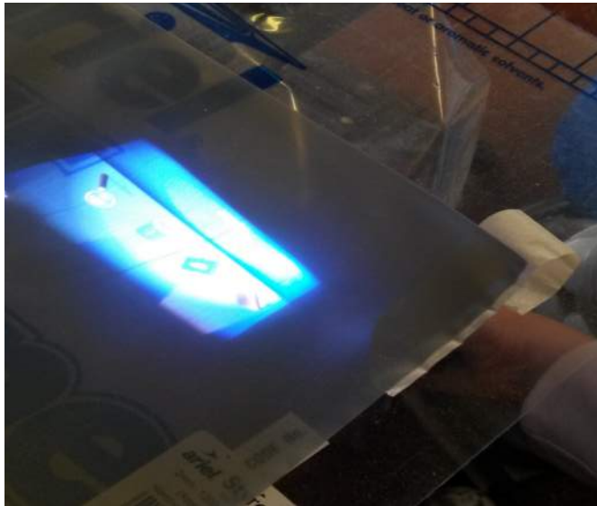
Step 13: The projection was accomplished using a projection material called Rear Projection sandwiched between the perspex.
