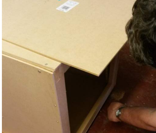
Step 8: A floor was then put in easily by slipping into place on the inside giving it a tight fit.
