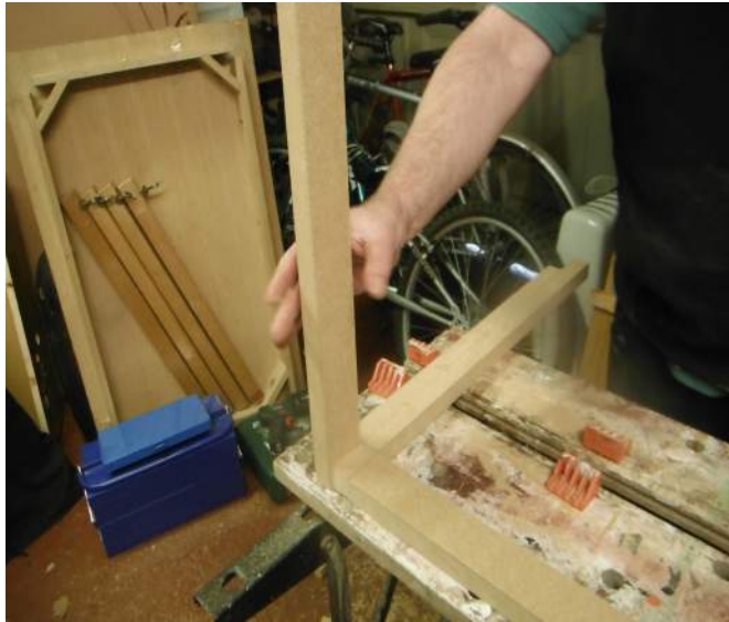
Step 2: The next step was to create the frame this was done using the timber beams which were screwed together.
